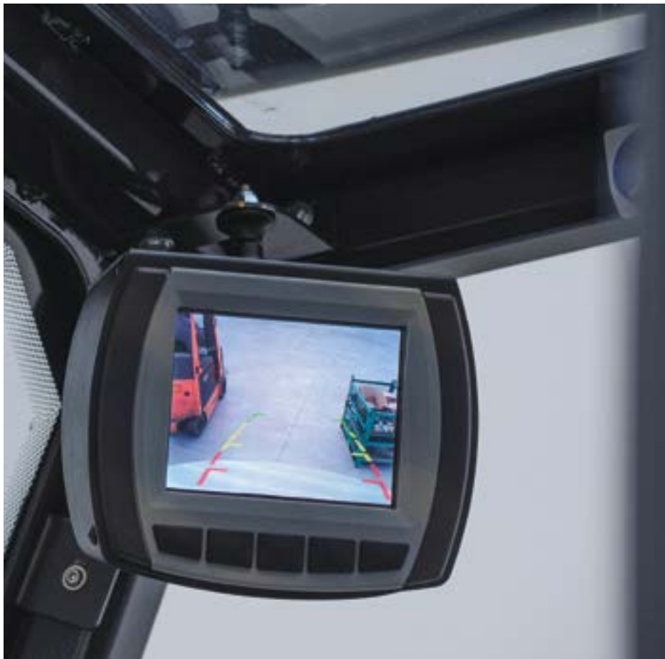
LEFT: The Curtis enGage vehicle display instrument used as a reverse safety camera
