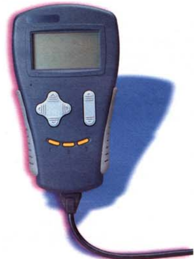
The CAN-compatible Curtis Model 1311 programmer for setting parameters and performing diagnostic functions
