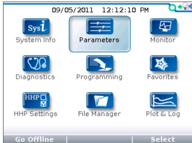
In the Main Menu, highlight the Parameters icon and press the “Select” softkey to go to the Parameters menu. You can return to the Main Menu at any time by pressing the Main Menu key (☐).
