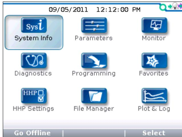
In the Main Menu, highlight the System Info icon and press the “Select” softkey to go to the System Info menu. You can return to the Main Menu by pressing the Main Menu key (☰).
