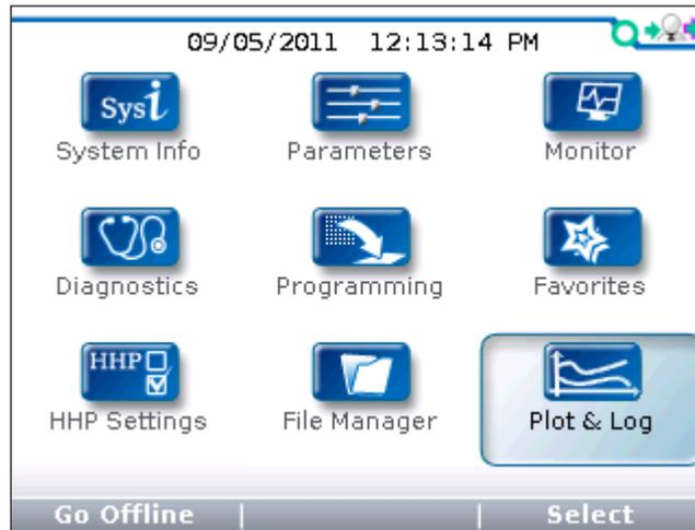
In the Main Menu, highlight the Plot & Log icon and press the “Select” softkey to go to the Plot & Log menu. You can return to the Main Menu at any time by pressing the Main Menu key (⏏).
