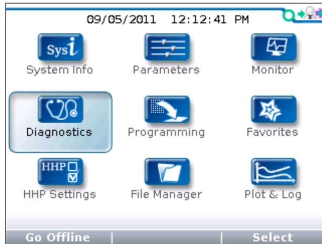
In the Main Menu, highlight the Diagnostics icon and press the “Select” softkey to go to the Diagnostics menu. You can return to the Main Menu at any time by pressing the Main Menu key (⌂).
