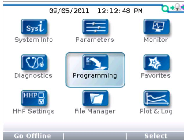
In the Main Menu, highlight the Programming icon and press the “Select” softkey to go to the Programming menu. You can return to the Main Menu at any time by pressing the Main Menu key (☰).
