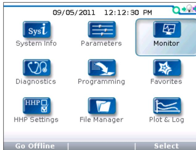
In the Main Menu, highlight the Monitor icon and press the “Select” softkey to go to the Monitor menu. You can return to the Main Menu at any time by pressing the Main Menu key (☰).
