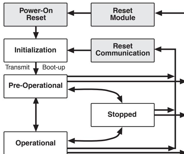
When the 1353 powers up, it goes to the Initialization state; this is also known as the Boot-up state. No CAN communications from the 1353 are transmitted in this state although the 1353 listens to the CAN bus. When the 1353 has completed its startup and self-tests, it issues an initialization heartbeat message and automatically goes to the Pre-Operational state.
