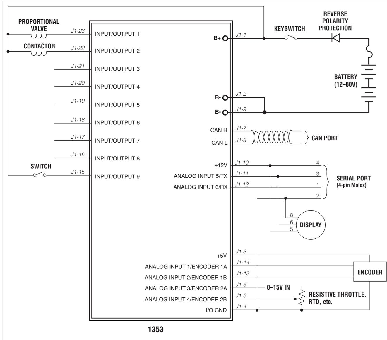
**Fig. 3** Basic wiring diagram, Curtis 1353 CANopen expansion module.
