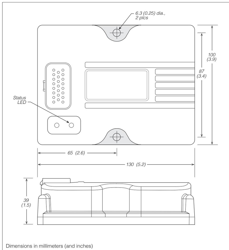
If the outputs will be used at or near their maximum ratings, it is recommended that the module be mounted to a good heatsinking surface, such as an aluminum plate.
