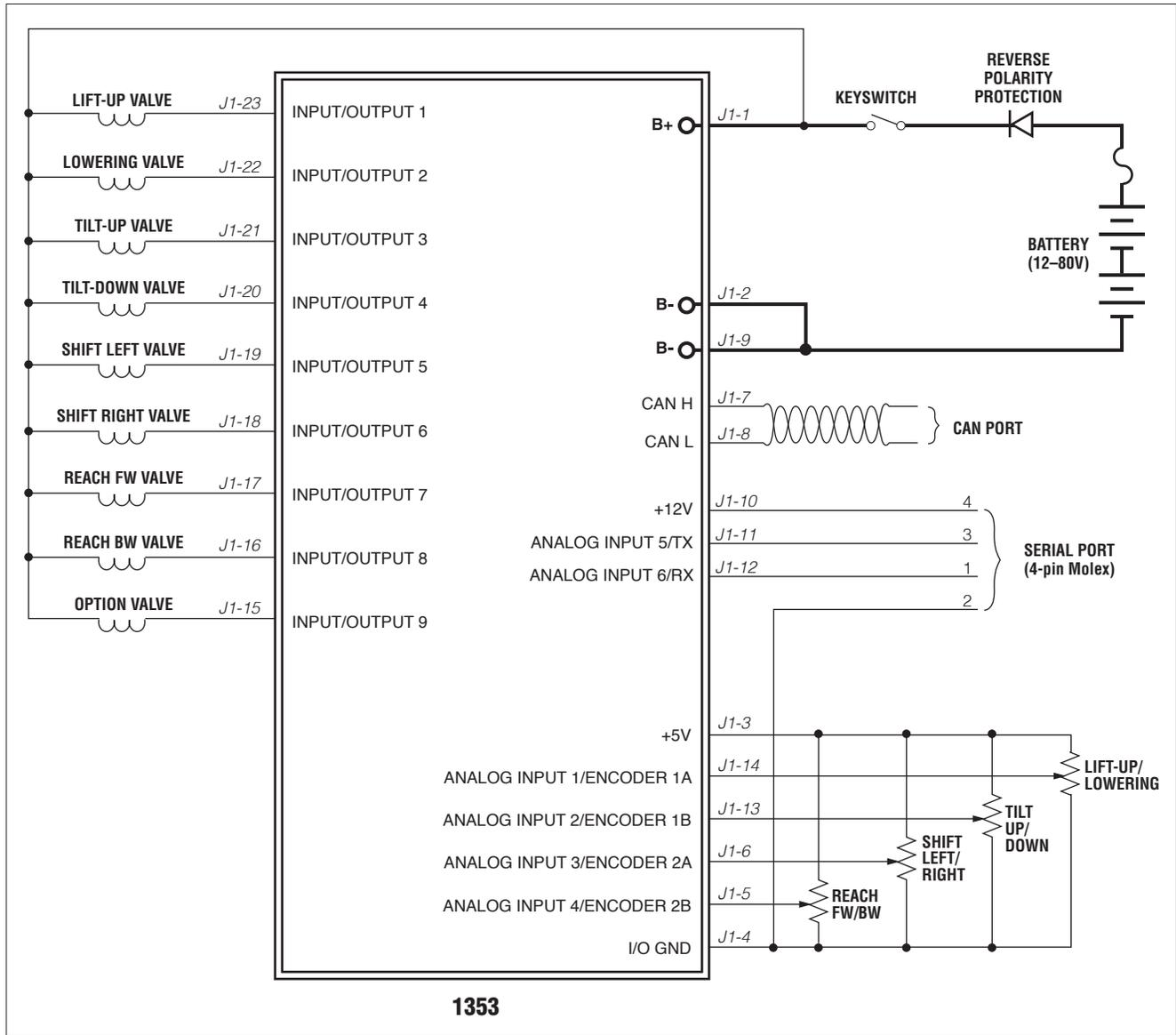
Fig. 4 Application example, Curtis 1353 CANopen expansion module.
